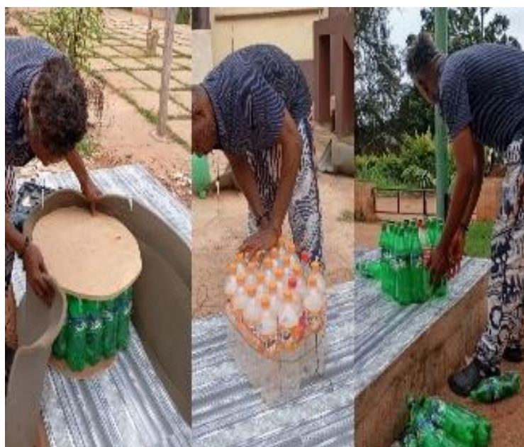
Plate 13. The researcher constructing eco-friendly stage furniture with plastic bottles Photograph by researcher.
