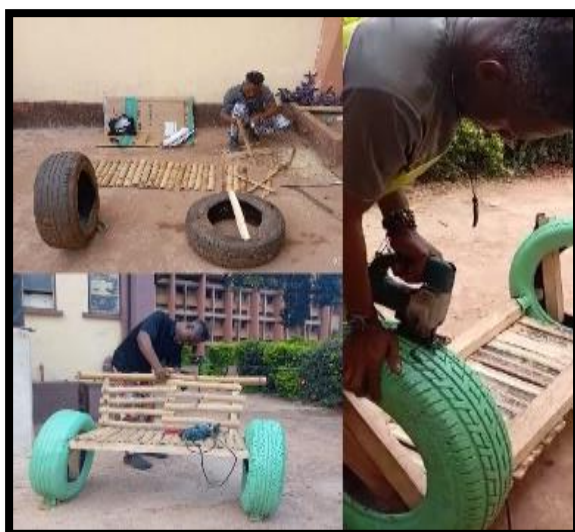
Plate 11. The researcher constructing mobile scenic unit from reclaimed tyres & bamboo. Photograph by researcher.
